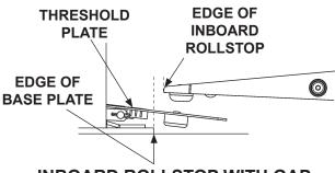
**INBOARD ROLLSTOP WITH GAP BETWEEN BASE PLATE** FIG. 53-2
